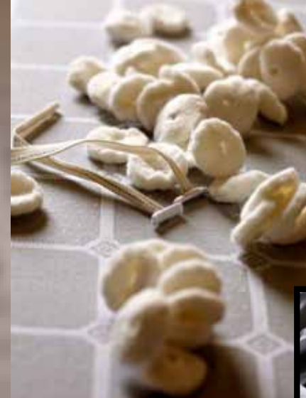
(Left and centre left) Cotton tufts linked by tapes are used to finish each mattress; they are positioned by hand using a long needle. (Below) The leather label denotes the bed model; the dark grey label is signed on the underside by the person who made the bed. (Right) Vernam Brown, known as TJ, stitches a mattress seam. (Bottom left) Rodica Grigoriu cuts Savoir's trademark ticking, designed by Richard D'Oyly Carte's wife Helen in 1905.
