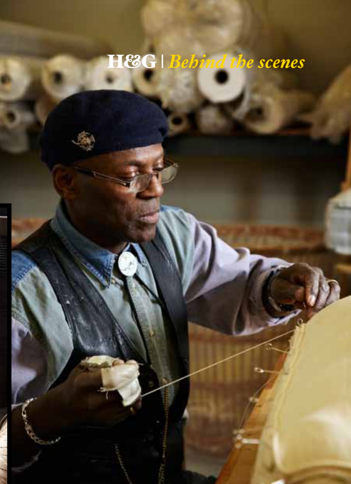
(Left and centre left) Cotton tufts linked by tapes are used to finish each mattress; they are positioned by hand using a long needle. (Below) The leather label denotes the bed model; the dark grey label is signed on the underside by the person who made the bed. (Right) Vernam Brown, known as TJ, stitches a mattress seam. (Bottom left) Rodica Grigoriu cuts Savoir's trademark ticking, designed by Richard D'Oyly Carte's wife Helen in 1905.
