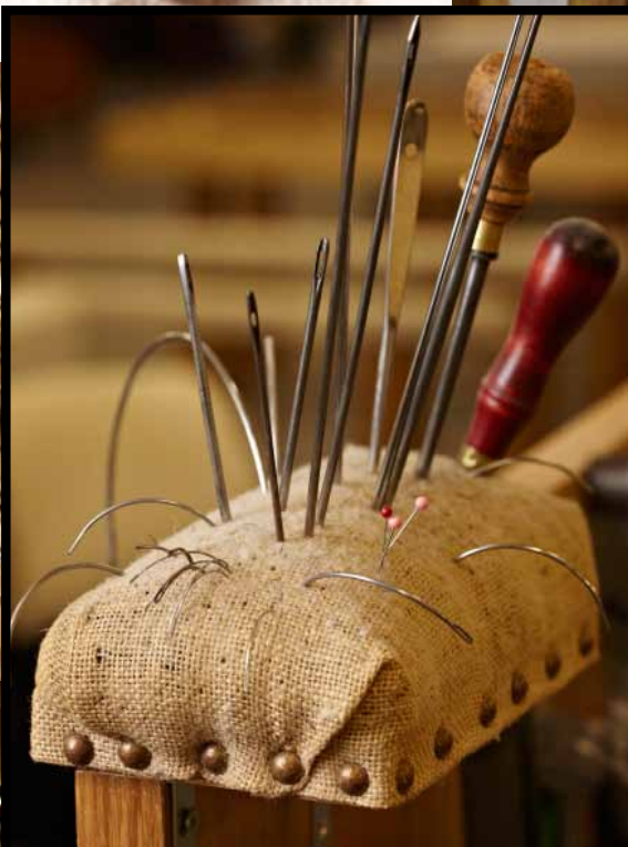
(Top left and above) Some of the traditional tools and needles used to make Savoir beds. (Top right) Each mattress is made by one person from start to finish. Lambswool and curly horse tail are valued as padding. (Right) Making a headboard is a painstaking process – here craftsman Dennis Taiwo tacks lining fabric to the back. (Centre left, top) Hourglass springs are tied together to ensure independent movement. (Left) Individual pocket springs in calico cases form the core of a Savoir mattress. ▶
